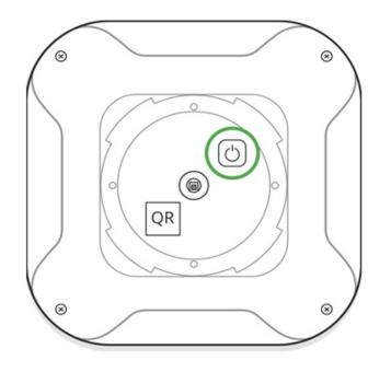
To make sure that the detector is on, press the on/off button — the logo will light up red for a second.
