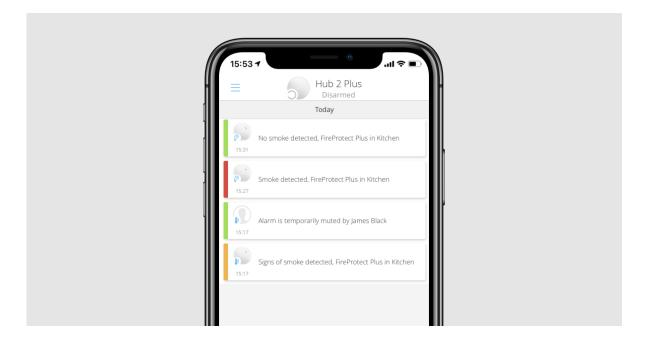
4. An alarm confirmation event is sent to the monitoring station and security system users, and the system starts the interconnected alarm for fire detectors if:
