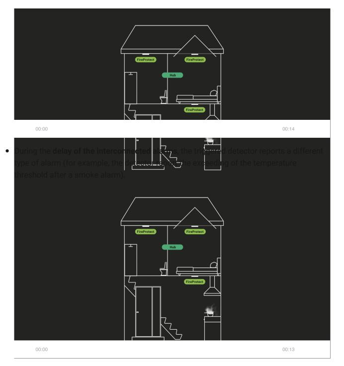
• During the **interconnected alarm delay**, another fire detector in the system raised an alarm.
